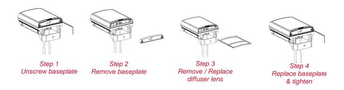
The illuminator is delivered with a 35° beam angle. To alter to 10°, remove the baseplate from the bottom of the product and remove the existing lens and then reattach the baseplate securely. With no lens insert the product produces a 10° beam angle.
