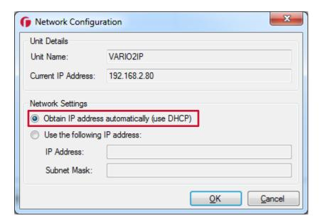
The unit will now be allocated an IP Address via the networks DHCP server. Refresh the RayLED Discovery Tool by pressing *Discover*. The illuminators IP address should automatically be updated into the required range and the illuminator can now be accessed directly from the RayLED Discovery Tool by double clicking on the illuminator from the list of discovered illuminators.
