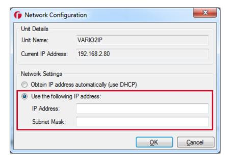
The unit will now be allocated the IP Address as entered. Refresh the RayLED Discovery Tool by pressing **Discover**.
