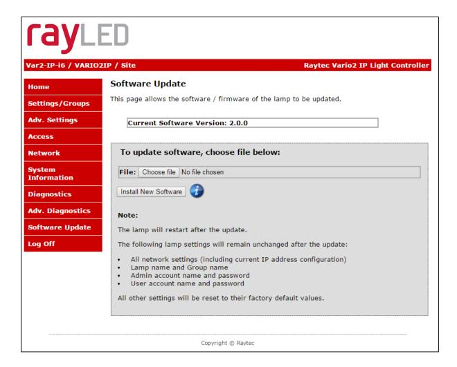
To upload a new version of software / firmware, please contact RayLED to receive the latest version.
