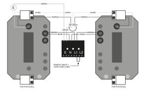
Typical wiring diagram - emergency luminaires
